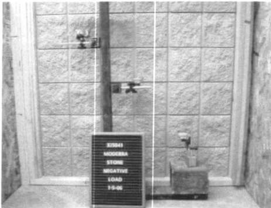
Typical Test Set-up for Moderra Stone (Negative)
